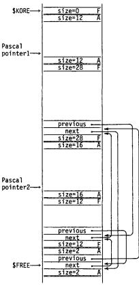
The boundary-tag scheme uses two additional words of storage to mark the boundaries of each block; lower and upper boundary words are identical. Each boundary word contains the size of the block and a one-bit tag that signifies whether the block is allocated or free. Since the size is always an even number of bytes, bit zero can be used to tag the block. Bit zero is clear to indicate that the block is free and is set to indicate that the block is allocated. Dispose need check only the boundary
